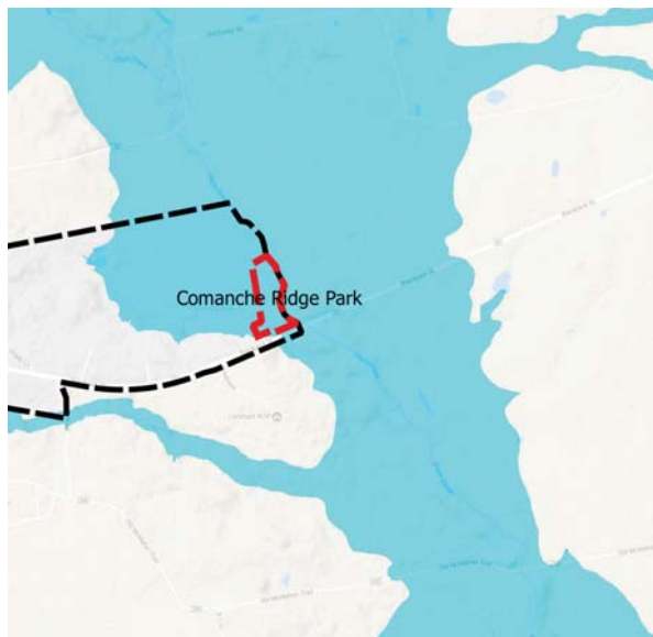
The Comanche Ridge Park property resides entirely within the floodplain (shown left) with a 1.0% Annual Chance of Flooding. This lends the property to being minimally developed for passive recreation uses.
