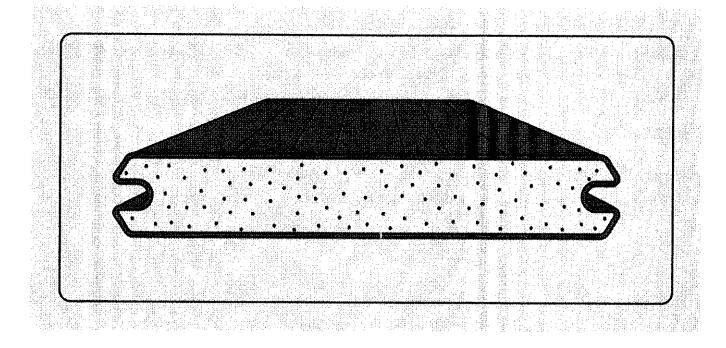
Manufactured decking includes composite and PVC materials that feature protective polymer caps. Boards may have three- or four-sided caps depending on the manufacturer and quality. Four-sided caps are the most protective since they prevent moisture penetration from every direction.
